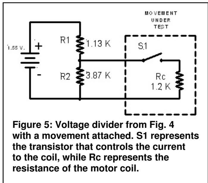
Now, as long as the coil remains disconnected from the circuit, the output voltage from the divider remains at 1.2 volts. When the switching transistor in the movement fires and connects the coil to the circuit, suddenly we have the coil's 1.2K resistance in parallel with R2, as shown in Figure 6. This changes the resistive values in the voltage divider, where the total resistance  $R_t$  is now equal to R1 plus the combined parallel resistances of R2 and Rc.
