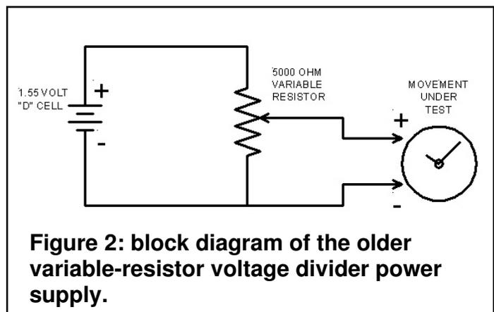
**Figure 2: block diagram of the older variable-resistor voltage divider power supply.**
