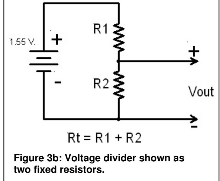
**Figure 3b: Voltage divider shown as two fixed resistors.**
