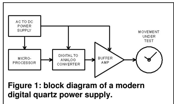
**Figure 1: block diagram of a modern digital quartz power supply.**
